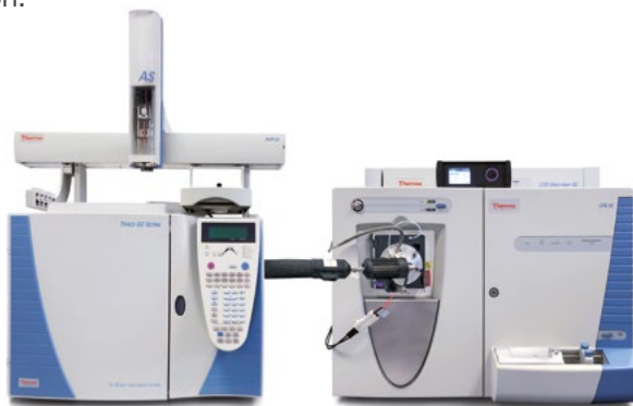
GC-SICRIT ® coupling to a high resolution LC-MS (e.g. TOF or Orbitrap platforms) for non-target screening with unmatched selectivity and accuracy.
