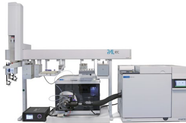
GC-SICRIT ® coupling to an LC-MS triple quad for routine quantification based on MRM workflows in e.g. pesticide analyses.
