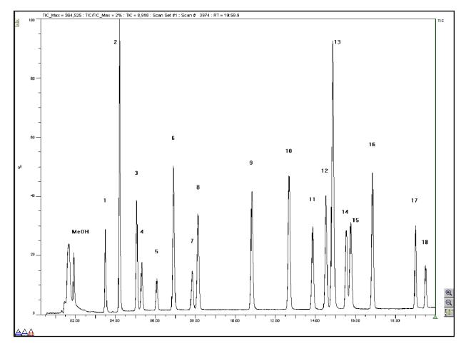
Figure 1. Chromatogram of the 19 Analytes in the VOC Specialty Mix at 5.0 ppb
