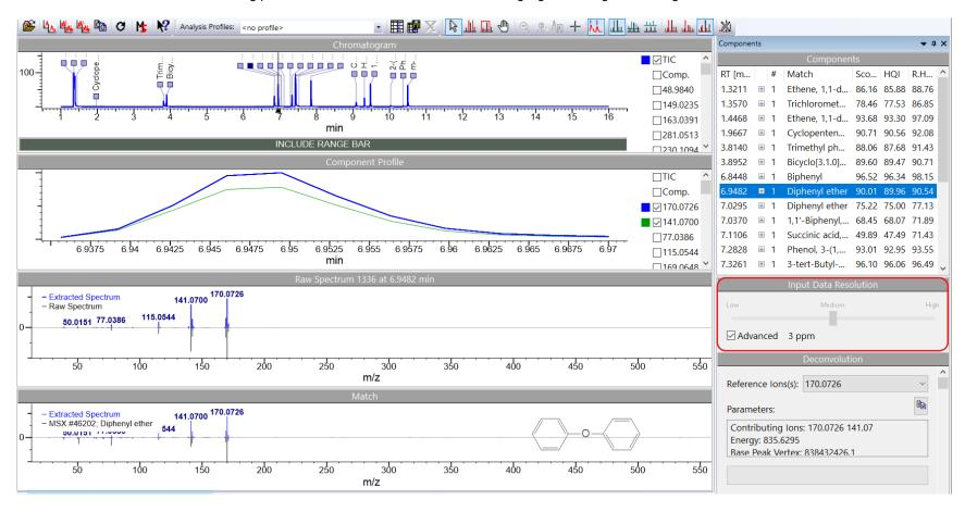
It is possible to save it as part of a profile, which can then be selected depending on the type of instrument. A user can create several profiles with different resolution settings for different types of data (and instruments).
