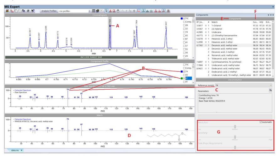
A – deconvoluted GC peak which found matches from reference MS databases; B – selected ions in a component; C – reference ion(s) used to model a component; D – extracted spectrum (top) vs reference spectrum (bottom); E – components table; F – combined spectrum search and reverse search Hit Quality Index (HQI) and, not shown in the above screenshot, each component's GC area under curve (AUC) value; G – Adjustable parameters in algorithm.
