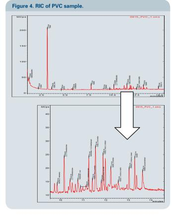
The compounds were tentatively identified and are listed in Table 3. Lower display is magnification of peaks eluting between 10 and 14 min.
