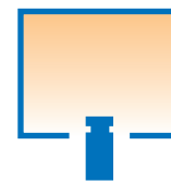
HS-20 Conveyance from the bottom makes it difficult for heat to escape from inside, improving oven temperature stability. (Patent US 8806965)
