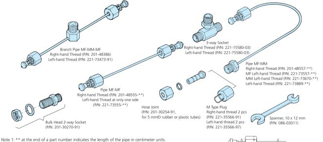
For details, please contact your local Shimadzu representative. Note 2: Left-hand thread of the pipe for hydrogen has a slit as a mark. Please refer to the figure at right.
