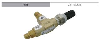
This valve is used to control the gas flow rate. The control range is 0 - 0.7L/min for nitrogen under an inlet pressure of 300 kPa. Shimadzu M type joints are used at both the inlet and outlet.
