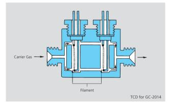
TCD must be pre-installed in a Shimadzu factory. Otherwise, the specified noise level and sensitivity cannot be guaranteed.
