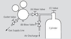
The air purge system consists of two valves, A and B. Close valve A and replace the cylinder, then open valve B and the cylinder valve C to discharge the air. Then close valve B and open valve A. By following these steps, carrier gas containing no air is supplied.
