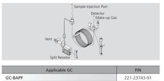
CLH-800 enables using the split injection method in a GC-8A system. Three types of split ratios are available depending on the type of resistors.
