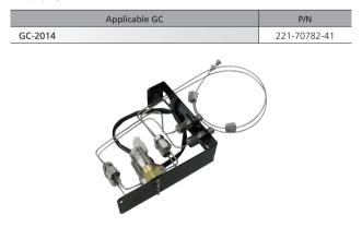
This Solenoid Valve Unit is connected to the detector's supply gas (hydrogen, air). It not only can shut off the supply gas according to instrument power supply or system ON/OFF operation, but also enables automatic start up and shutdown after analysis ends. Therefore, the supply gas can be shut off during a power outage to ensure a safer laboratory. Flame status can also be monitored in GC-2014.
