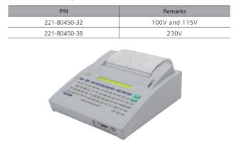
The easy-to-use C-R8A includes various peak processing functions and quantitative calculations, making it suitable for routine work in quality control laboratories. C-R8A has an automated validation function to support GLP/GMP/ISO requirements, and is equipped with a high-speed RS-232C port (19,200 bps) for a network system using CLASS-Agent or Chromatopac manager software programs.One formatted SD card is included.
