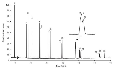
Figure 2: TIC chromatogram for 10  $\mu$ g/mL 18 component PAH mixture on an equiv 5SilMS phased 30 m × 0.25 mm × 0.25  $\mu$ m GC column
