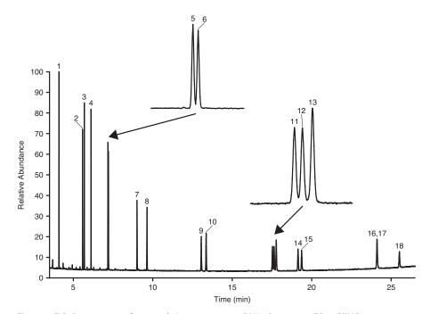
Figure 1: TIC chromatogram for 10  $\mu g/mL$  18 component PAH mixture on a TG-17SilMS 30 m  $\times$  0.25 mm  $\times$  0.25  $\mu m$  GC column
