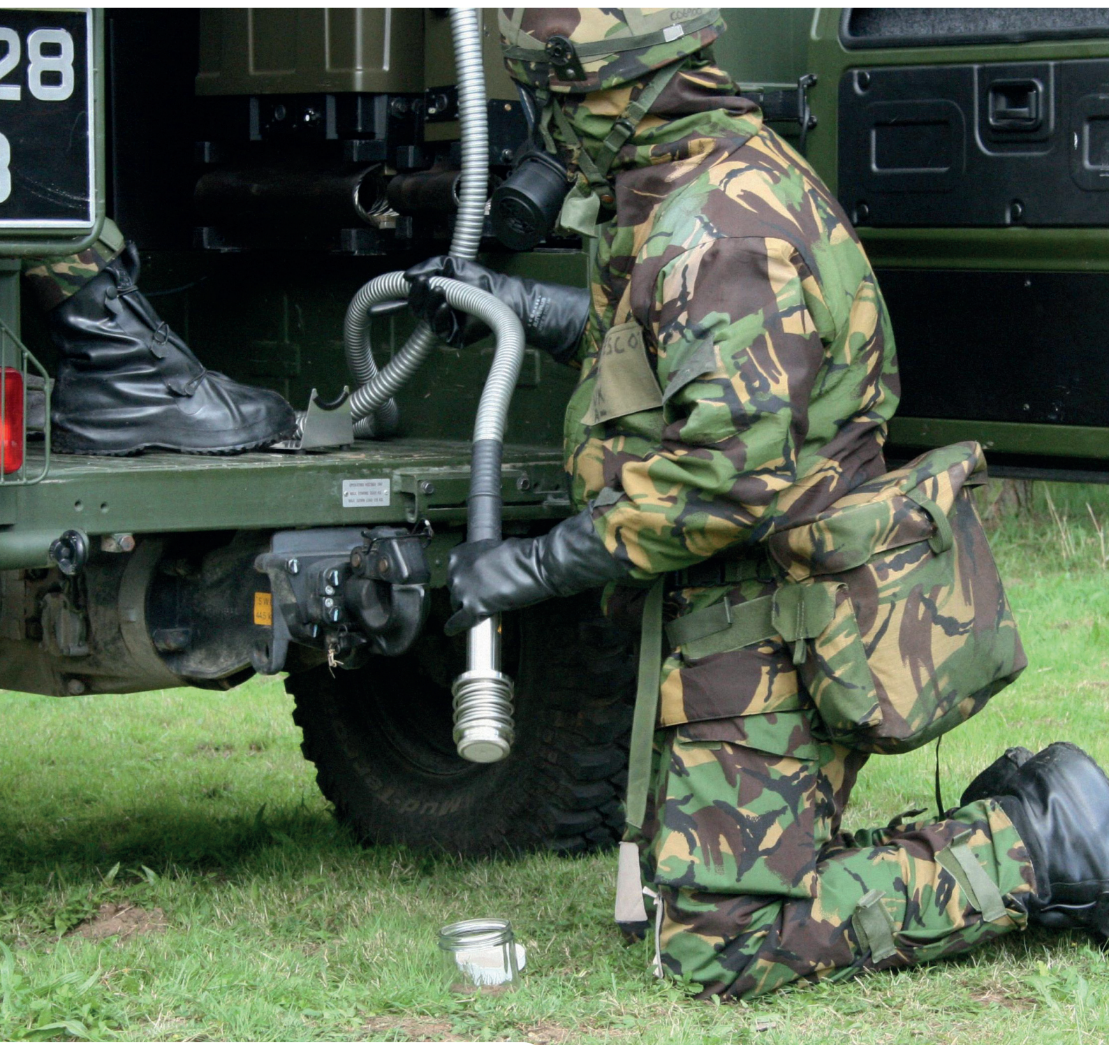
The Bruker MM2 is used to test soil for the presence of CWA.
