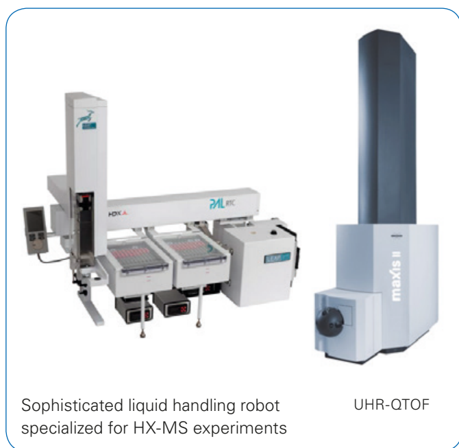
Fig. 1 Key components of the robotic setup for automatic HX-MS experiments
