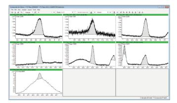
Figure 6. An 85  $\mu m$  CAR WR/PDMS Fiber MDL replication (BTEX targets shown).
