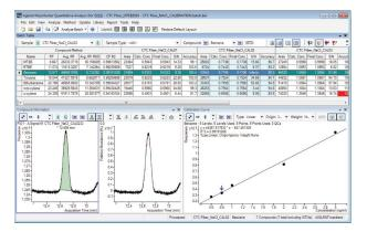
Figure 4. MassHunter Quant Batch view of 85  $\mu m$  CAR WR/PDMS Fiber calibration (benzene shown).
