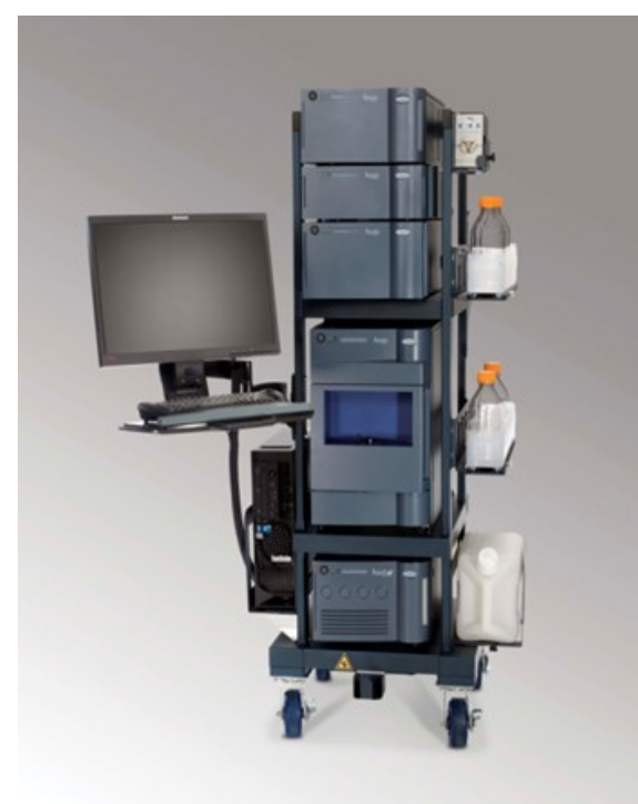
Figure 3. System components of a PATROL UPLC Pilot Process Analysis System on the PATROL Pilot cart
