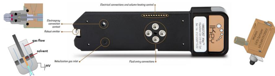
**Figure 2.** The electrospray design within ionKey high-pressure microfluidic device was incorporated to improve DESI sprayer. Briefly, stainless steel emitter recessed behind critical orifice, nebulization gas sheathes primary solvent to create liquid jet. Schematic representation of prototype sprayer is shown on the right.
