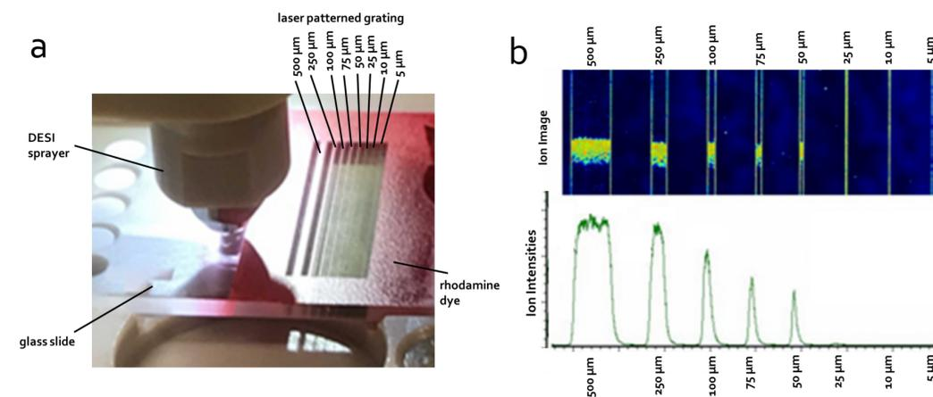
**Figure 4.** (a) Precision laser etching was used to create pattern with defined spacing, from 5  $\mu$ m to 500  $\mu$ m over rhodamine dye coating; (b) images at the defined grating is shown on top, the image at 10  $\mu$ m and 5  $\mu$ m are may be below of limit of detection, the ion intensities for each spaces grating is shown below.
