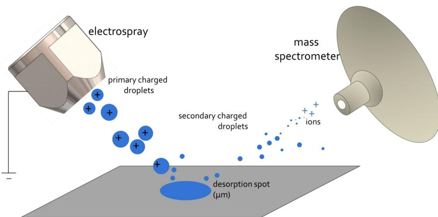
**Figure 1.** DESI MS is performed by extracting and ionizing, in-concert, from a sample surface. Briefly, primary droplets produced by the sprayer forms a thin film of solvent at the surface extracting analyte molecules off tissue, the subsequent primary droplets colliding with the film generate secondary droplets that are ejected, desorbed, ionized, and analyzed by mass spectrometer.
