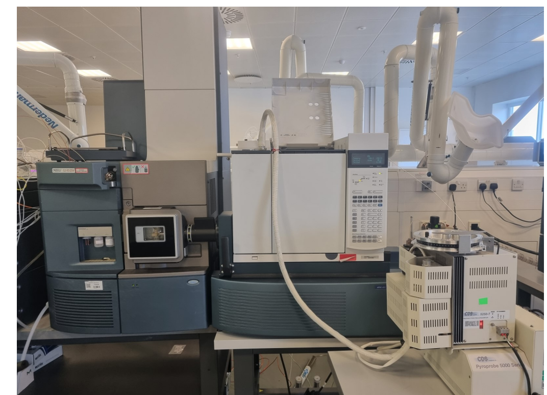
Figure 1. Pyrolyzer coupled to the APGC QToF mass spectrometer.
