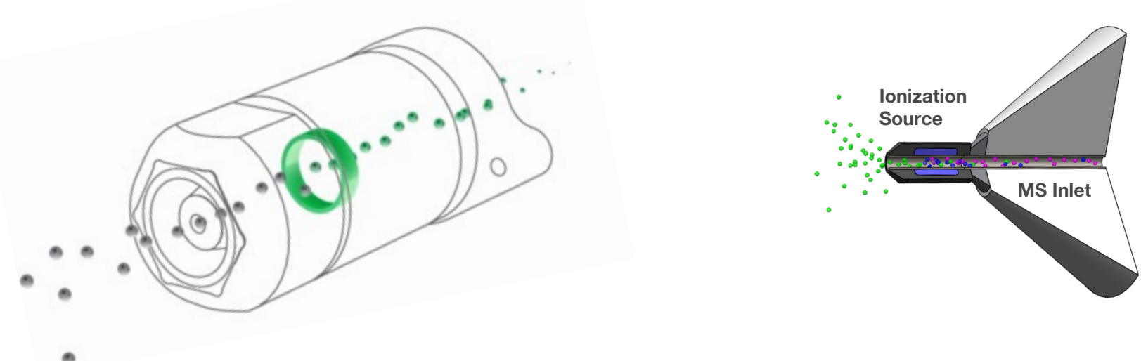
Figure 1: Schematic diagrams of the SICRIT source with plasma-based core (left) and attached to an atmospheric pressure MS (right)
