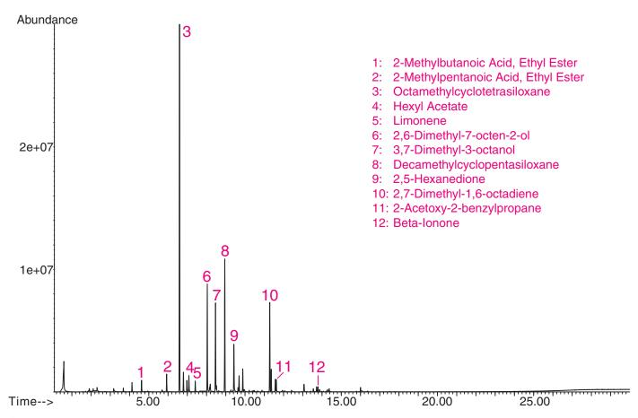
**Figure 3.** Total Ion Chromatogram resulting from Direct Thermal Extraction.
