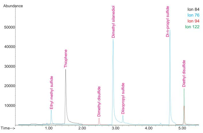
Figure 2. Chromatogram of sulfur compounds in IPA.
