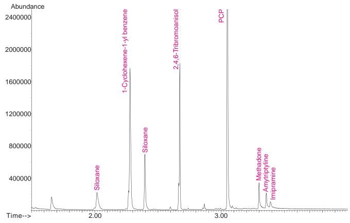
**Figure 7.** Chromatogram for 1<sup>st</sup> extraction of saliva.
