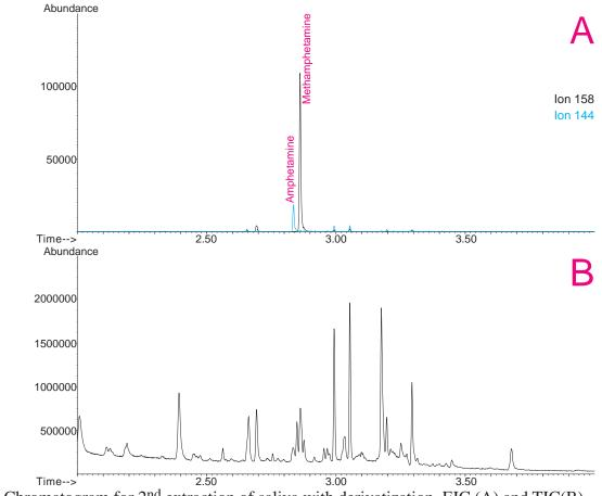
Figure 8. Chromatogram for 2<sup>nd</sup> extraction of saliva with derivatization, EIC (A) and TIC(B).
