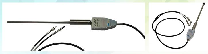
The industrial immersion probes on B&W Tek's portable Raman instruments feature a stainless steel probe body along with a stainless steel or hastelloy probe shaft. They are immersible in liquids, slurries, powders, and solids under pressure up to 6000 psi and temperatures up to 300 °C for hastelloy (200 °C for stainless steel).
