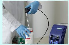
The standard probes on B&W Tek's portable Raman instruments (models BAC102-xxx and BAC100B) come with standard aluminum shafts that are 3" (76.2 mm) in length with a diameter of 0.371" (9.42 mm), operable up to 80°C for non-immersive use (model RSS100-xxx). In addition, the shafts on these probes are user-replaceable, giving the flexibility to adapt to different working environments.
