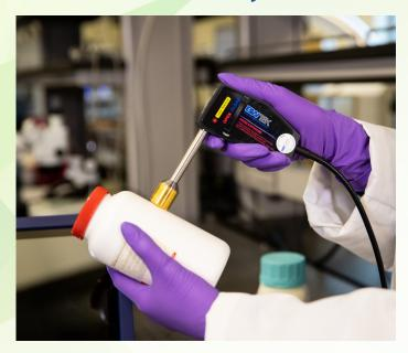
B&W Tek also offers a large area probe with increased penetration depth that can be used with our 785 or 1064 i-Raman Prime or PTRam systems. With the 4 mm diameter measurement area, bulk property measurements of heterogeneous samples can be made. These ST probes, when used with our BWID software, give the ability for see-through identification of material in opaque packaging.
