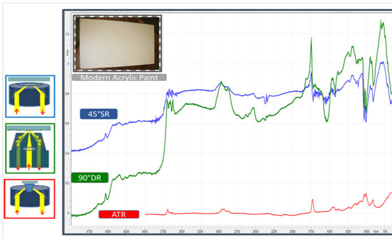
Figure 2. Spectra of a modern acrylic white paint collected by ATR (red), diffuse reflectance (green) and 45° specular reflectance (blue) interface FTIR measurement techniques. The left side bar illustrates the IR beam path of each interface type with color-coded box (red-ATR, green-diffuse reflectance & blue-45° specular reflectance)
