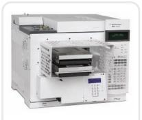
The Agilent LTM System consists of a replacement door for either the Agilent 7890 or the Agilent 6890 that has built-in electronics and slots for inserting from 1 to 4 GC column modules. Programming can be done via Agilent ChemStation software or using a simple keypad control user interface. Up to 10 methods may be stored.
