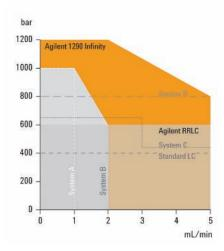
The power range of the Agilent 1290 Infinity LC is the widest available, combining ultrahigh pressures up to 1200 bar and high flow rates up to 5 mL/min for maximum chromatographic performance, compatibility, flexibility and investment protection.
