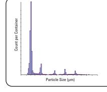
The 7080 AccuSizer, with its ability to count and size individual particles, is a sensitive tool for constructing a material's true particle size. Here, five latex standards of varying size were used in a single sample; all were successfully located by Agilent's 7080 AccuSizer.
