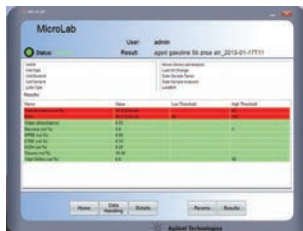
Note: Aged Gasoline, EtOH, Light Aromatics, and Light Aliphatics Evaporated, Measured on the Multireflection 5500a Gasoline Method
