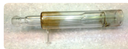
Figure 1. Torch in need of cleaning
