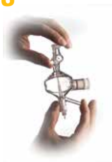
Multi-mode Sample Introduction System (MSIS) for sub ppb detection of As, Hg and Se
