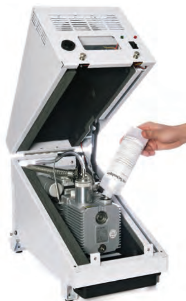
Quiet Cover GC/MS, with open-access cover
