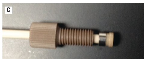
Figure 1. Installation of PEEK tubing from solvent bottles to pump.
