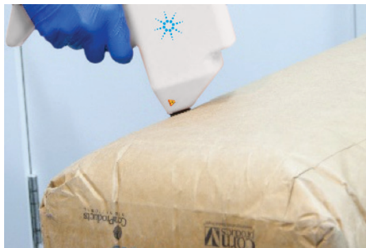
Raw material identity verification through a multilayer paper sack.
