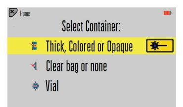
Figure 1. Selections for through-barrier, point-and-shoot, or glass vial measurements.
