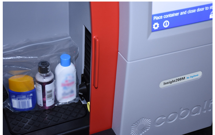
Figure 4. Screening a 100 mL container while still inside a 1 L plastic bag.
