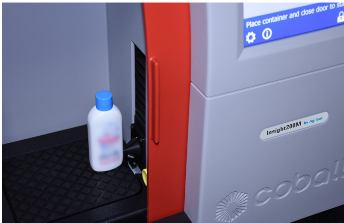
Figure 3. Screening a 100 mL container in an Insight200M system.
