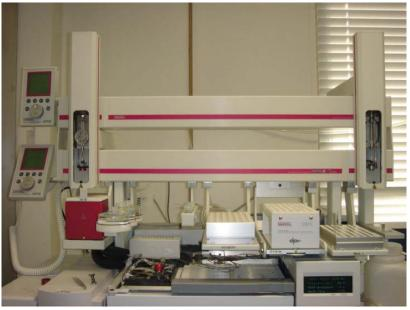
**Figure 1.** A picture of the dual rail GERSTEL MPS 2 with DPX automation platform. The left MPS is equipped with a 100 uL syringe for injecting eluent and derivatizing reagents, and the right MPS is equipped with a 2.5 mL syringe for performing DPX extractions.
