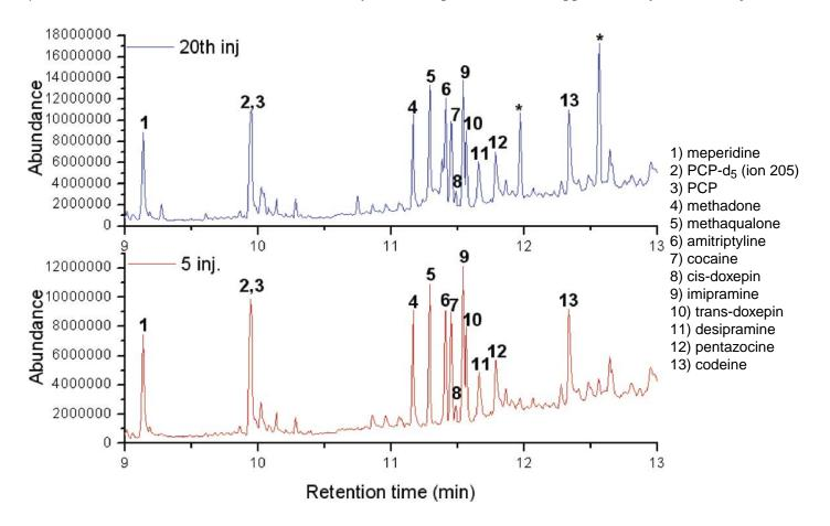
**Figure 2.** Total ion chromatograms of basic drugs extracted from 0.25 mL of whole blood spiked at 0.5 ppm. The top chromatogram represents the 20th large volume injection of 50  $\mu$ L of whole blood extracts, and the bottom chromatogram represented the 5th injection. \*-Denotes septum bleed from the vial cap from multiple injections.
