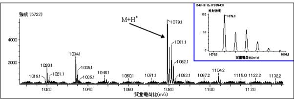
Top: ESI mass spectrum of NCP-Zn Bottom: Cold-spray mass spectrum and isotopic simulation mass spectrum of NCP-Zn
