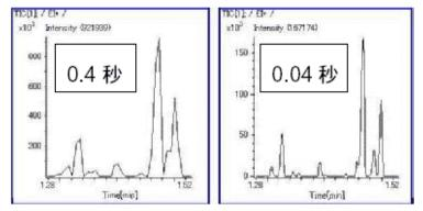
Figure 2. Chromatogram peak analysis in fast GC at different recording speeds (Left: 0.4 sec; right: 0.04 sec; both acquired in AccTOF GC)
