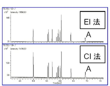
Figure 1. TIC of liquid crystal (top: EI; bottom: CI)
