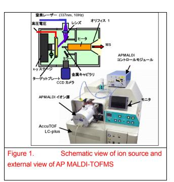
capillary up to 400°C, efficiently directing the ions from atmosphere to high vacuum. The ion source, in atmosphere, allows for speedy loading and unloading of the sample plate. The ion
