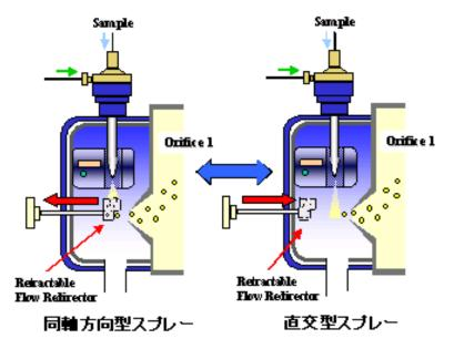
Vertical gas flows from the sprayer are effective in minimizing contamination buildup in the MS system. For some samples, however, ionization efficiency is often inferior to coaxial gas flows.
