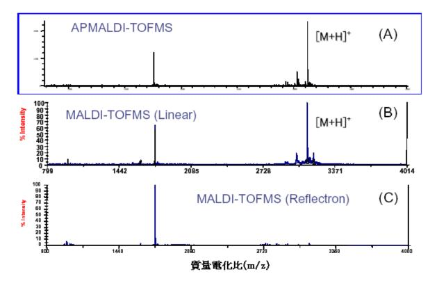
Figure 2. MS spectra of β-casein (bovine) fragment 1-25 acquired in AP MALDI-TOFMS (A), Linear mode of MALDI (B), and Reflectron mode of MALDI (C)
