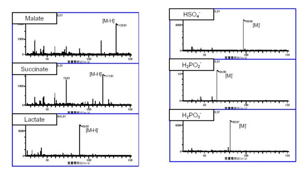
Figure 2. Mass spectra of anions in Sample (1)
