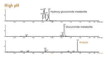
With ACQUITY UPLC and BEH column technology, we were quickly able to determine that high pH yielded the best resolution of two coeluting metabolites of our analyte.
