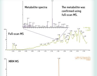
The novel collision cell design of the Xevo TQ MS, where the collision gas is always on, allows for simultaneous collection of full-scan MS and MRM data in a single analysis, without compromising speed, and with no loss in MRM sensitivity. You collect both qualitative and quantitative data in one run.
