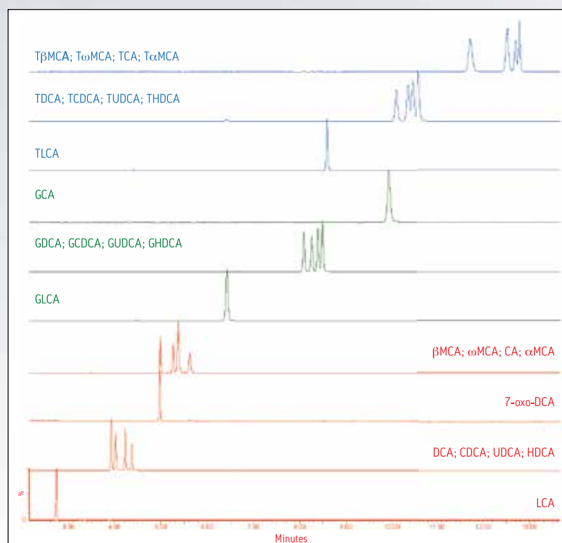
Figure 1. Simultaneous analysis of a 25-bile acids standard mixture including glycine and taurine conjugates was achieved within 13 minutes. The compound name is shown in order of retention time on each MRM chromatogram.
