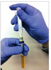
Figure 1. Oasis PRIME HLB Cartridge used in pass-through cleanup of a QuEChERS spinach extract.
