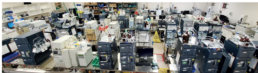
Eurofins' laboratory in Des Moines includes more than 50 Waters LC instruments with optical detectors.
