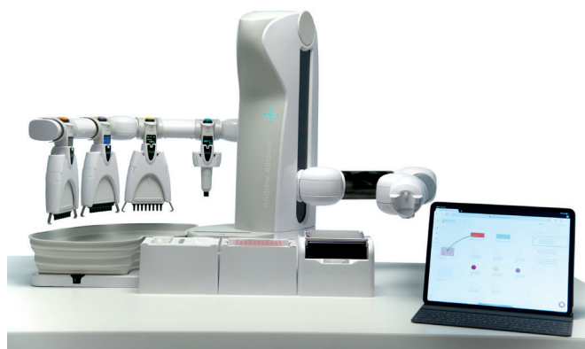
The Eurofins team trialed the Andrew+ pipetting robot to improve efficiencies in the lab.
