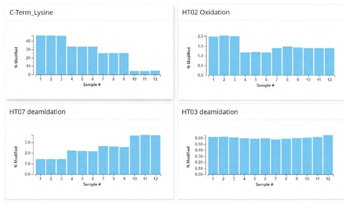
Figure 5. Bar graphs showing results presented in the Peptide MAM App for four monitored attributes, C-terminal Lysine, HT02 oxidation, HT07 oxidation, and HT03 deamidation. Injections are labeled as 1–3 for Remicade, 4–6 for Inflectra, 7–9 for Avsola, and 10–12 for Renflexis.
