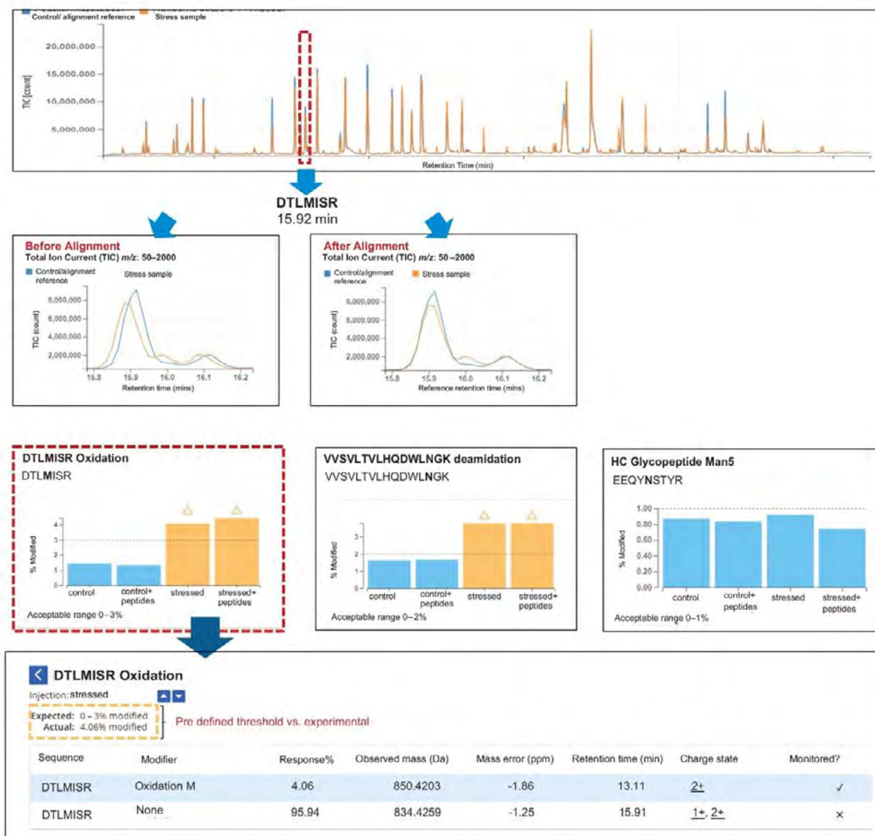
Figure 5. The retention time alignment panels (A) show the pre- and post-alignment of the DTLMISR peptide peaks from the control and alignment reference samples as an overlaid chromatogram. The monitored attribute peptide panel (%Abundance) is displayed for three modified (oxidized, deamidated, and glycosylated) peptides. Predefined pass/fail criteria based on user defined limits determine the color of bars, and the presence of a warning icon above them. The table, below, displays target criteria and results for the DTLMISR Ox attribute from the stressed sample.
