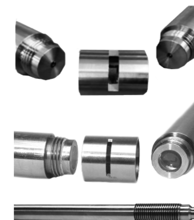
Top: Transmission probe pairs with spacer, top center: single fiber, middle center: microbundle fiber. Bottom center: Transmission pair with thread for implementation in extruder.
