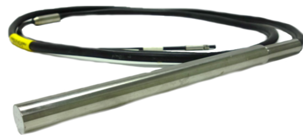
Non-contact probe used for the analysis of large non-uniform particles
