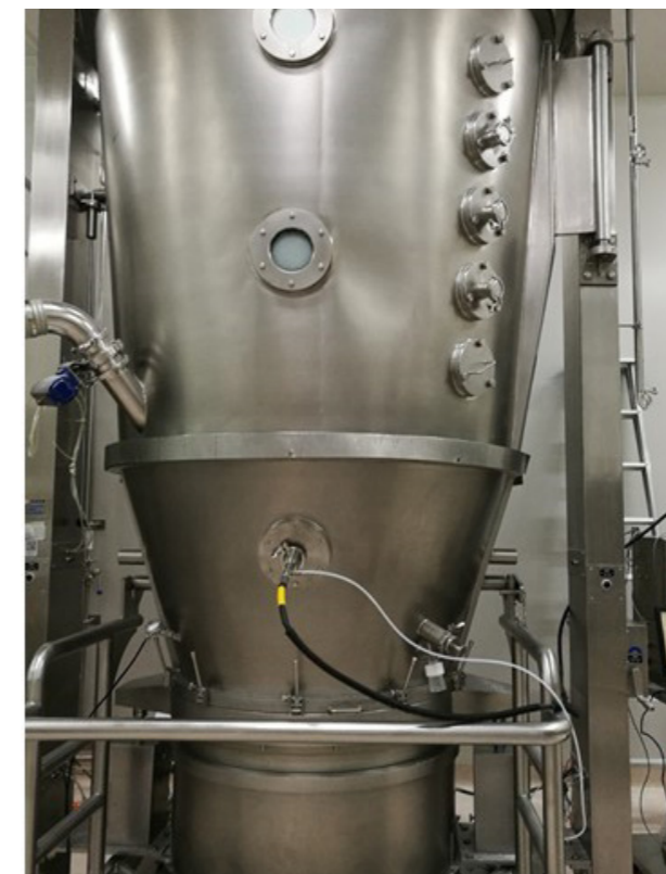
Spoon probe implemented in a dryer
