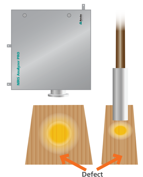
Illustration of the spot size difference between a NIRS Analyzer PRO and a non-contact probe
