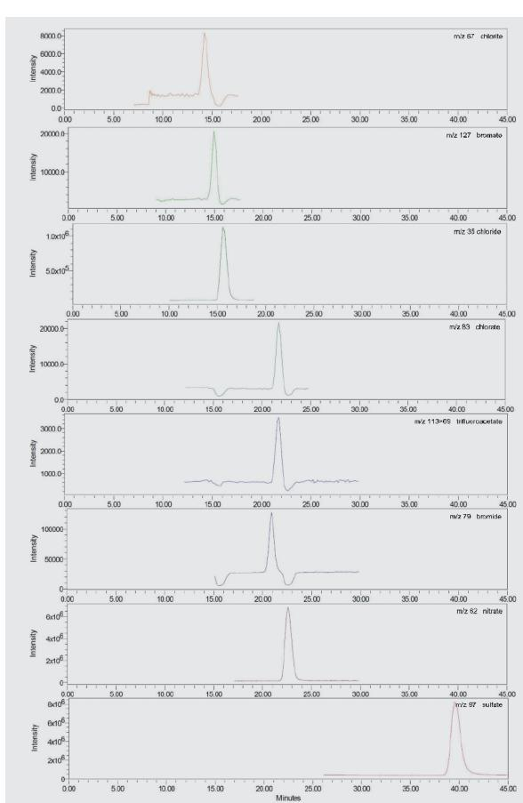
Conditions: 5 mg/L chloride, nitrate, sulfate, 0.1 mg/L bromide, 5 µg/L chlorite, chlorate, bromate, TFA; eluent: 3.6 mmol/L Na<sub>2</sub>CO<sub>3</sub> + 10% acetonitrile; flow rate 0.6 mL/min, injection volume 10 μL; 45 °C; sequential suppression; detection: conductivity & SIR (ES-)
