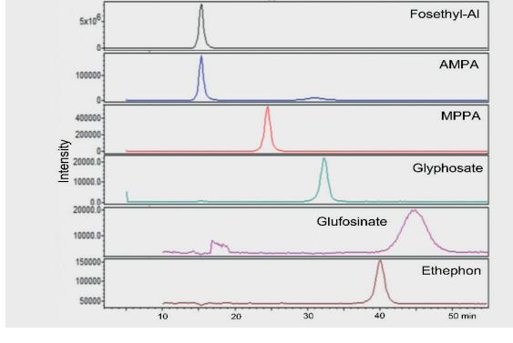
Eluent: (NH<sub>4</sub>)<sub>2</sub>CO<sub>3</sub>/NH<sub>4</sub>OH; 70/100 mmol/L, 30% isopropanol; flow rate: 0.3 mL/min; 32 °C; injection volume 200 μL; 32 °C; detection: SIR (ES-)
