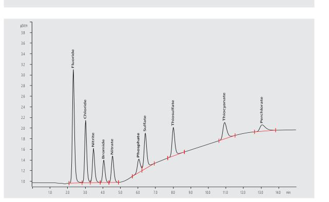
Anions and Oxoanions including thiosulfate, thiocyanate, and perchlorate were separated on a Metrosep A Supp 7 - 150/2.0 within 15 minutes. Conditions: 1 mg/L standard; eluent A: 3.6 mmol/L Na<sub>2</sub>CO<sub>3</sub>, eluent B: 20.0 mmol/L Na<sub>2</sub>CO<sub>3</sub>; flow rate: 0.6 mL/min; injection volume 10 μL; 55 °C; sequential suppression; detection: conductivity
