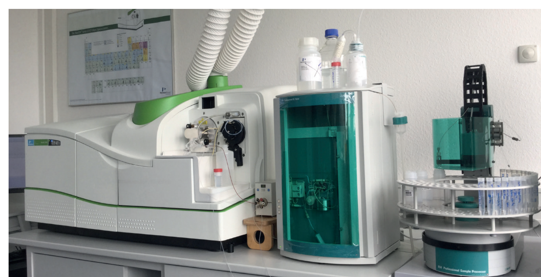
PerkinElmer NexION 350D ICP-MS (left) coupled to Metrohm Professional IC Vario One and Professional Sample Processor (right).
