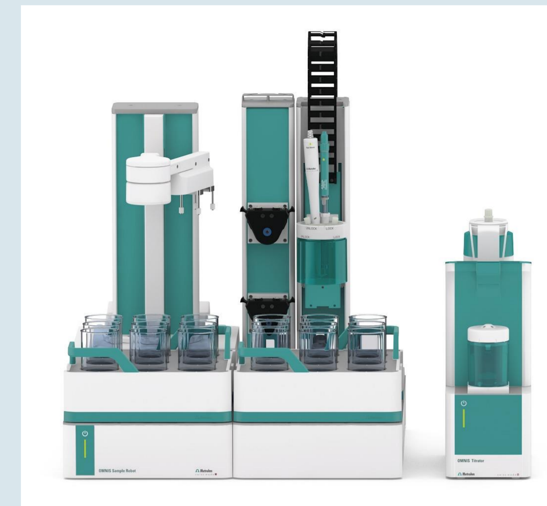
Fig 4: Autotitrator and electrode used for chemical medicine assay
