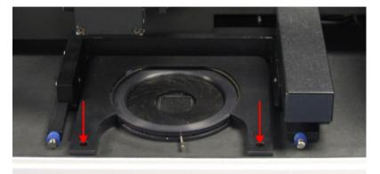
The pins hold the iris adapter securely in position over the sample window.
