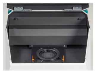
The pins hold the iris adapter securely in position over the sample window.
