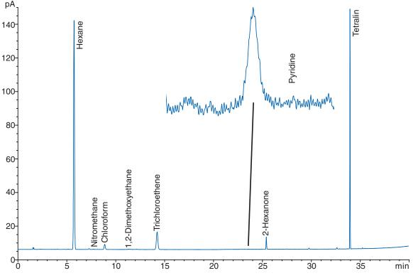
Figure 4. Chromatogram for the Class 2 mixture B standard solution on the Zebron<sup>TM</sup> ZB-624 column.
