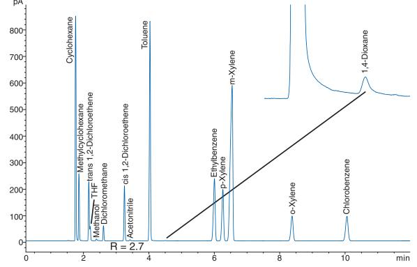
Figure 8. Chromatogram of the Class 2 mixture A standard solution on the Zebron<sup>TM</sup> ZB-WAXplus.
