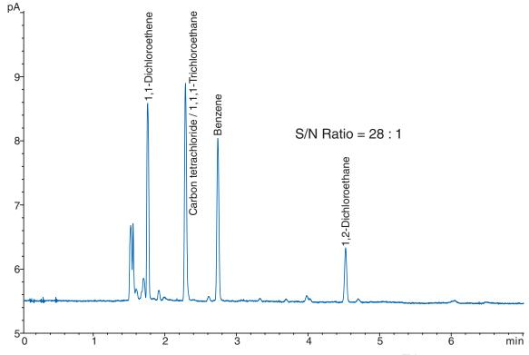
Figure 6. Chromatogram of the Class 1 system suitability solution on the Zebron<sup>TM</sup> ZB-WAXplus.
