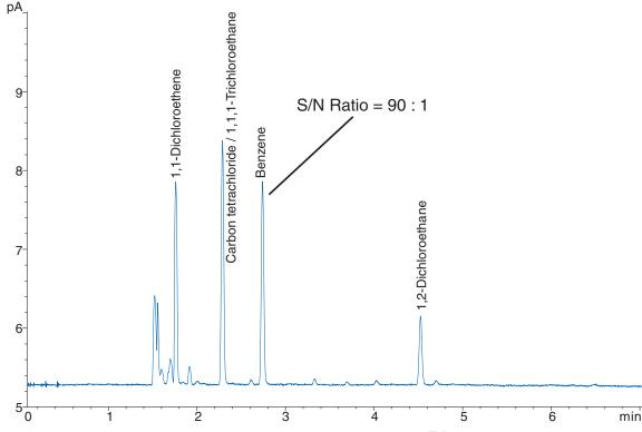
Figure 7. Chromatogram of the Class 1 standard solution on the Zebron<sup>TM</sup> ZB-WAXplus.
