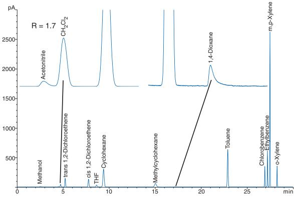
Figure 3. Chromatogram of the Class 2 mixture A standard solution on the Zebron<sup>TM</sup> ZB-624 column.
