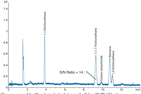
Figure 2. Chromatogram of the Class 1 standard solution on the Zebron<sup>TM</sup> ZB-624 column.
