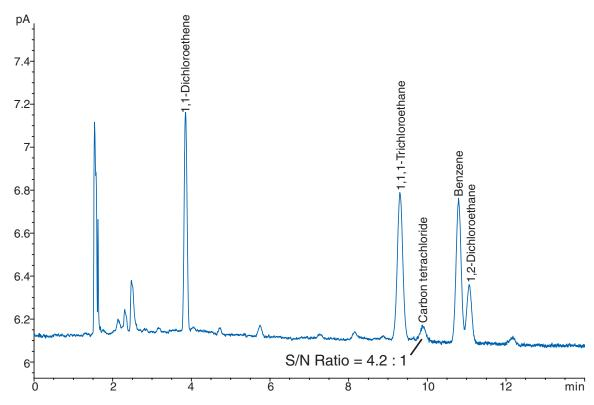
**Figure 1.** Chromatogram of the Class 1 system suitability solution on the Zebron<sup>TM</sup> ZB-624 column Figure 2 shows a chromatogram of the Class 1 standard solution with the 1,1,1-trichlorethane peak having a S/N ratio of 14.
