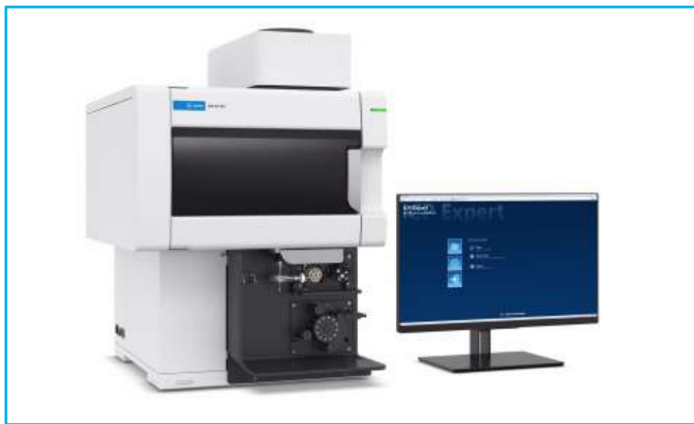
Figure 1. Agilent 5900 SVDV ICP-OES and ICP Expert software.
