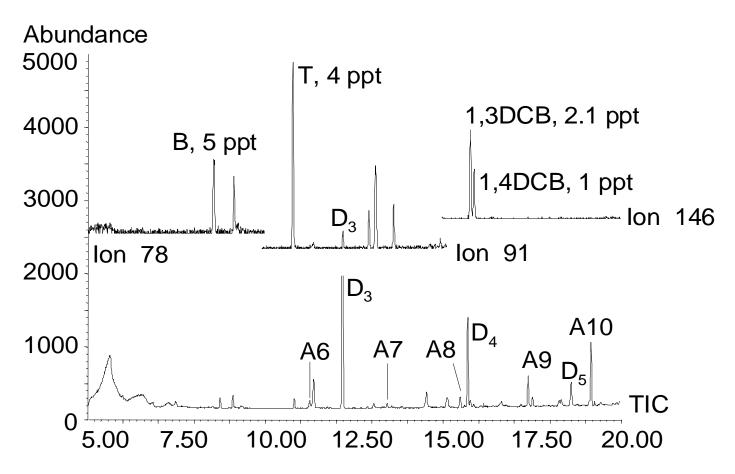
**Figure 4.** Analysis of surface sample by SBSE - thermal desorption - GC-MS (Peaks: B: benzene, T: toluene, 1,3-DCB: 1,3-dichlorobenzene, 1,4-DCB: 1,4-dichlorobenzene).
