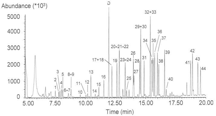
**Figure 3.** Analysis of water sample spiked with volatile priority pollutants at 2 ppb level using SBSE - thermal desorption - GC-MS.
