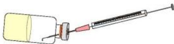
Figure 2: Schematic of the technique used to spike sample vials with water.
