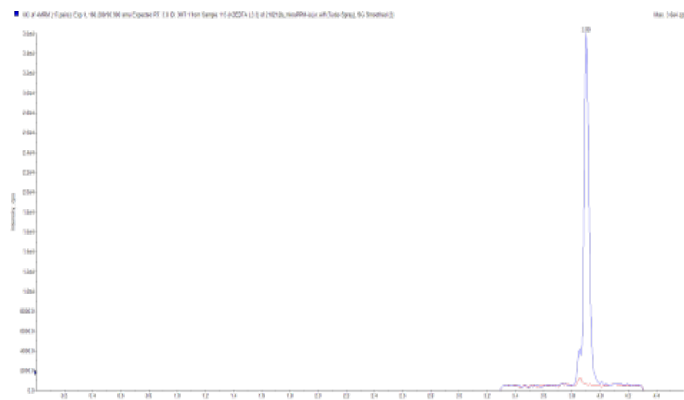
Figure 4. Extracted Ion Chromatograms, (80 pg mL -1 spiked potassium EDTA plasma, overlaid with stripped blank).
