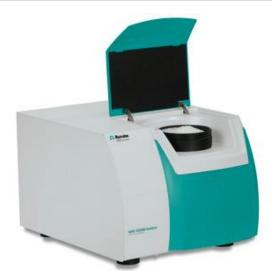
Fig. 1: A NIRS DS2500 Analyzer was used to collect the spectral data in reflection mode over the full wavelength range of 400 - 2500 nm. The large sample cup was used to average the spectral information taken at eight different spots of the polymer granulate.
