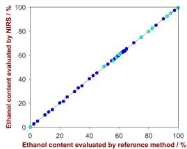
Fig. 4: Correlation plot of ethanol content predicted by NIRS versus reference values. A high correlation is observable. Displayed are the calibration (blue) and the validation data (turquois).
