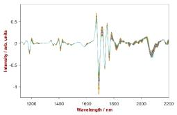
Fig. 3: 2- derivative spectra of 44 ethanol/isopropanol mixtures in the region of 1100–2200 nm.
