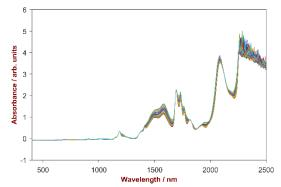
Fig. 2: Vis-NIR spectra of 44 ethanol/isopropanol mixtures.
