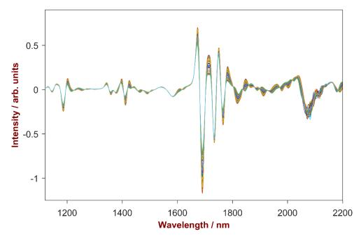
This Application Note describes a fast, nondestructive, and reliable method for the determination of the chemical composition of alcohol mixtures exemplified by ethanol/isopropanol mixtures. With visible near infrared spectroscopy (VIS-NIRS), results are available in real-time, thus making NIRS highly suited for fast quality control.
