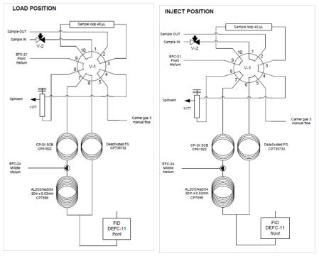
LPG's (Liquid Petroleum Gases) like propylene and all butane streams can be injected as a liquid through an optional liquid injection valve. In order to maintain sample integrity, a "pressure station" is recommended. The pressure station maintains a high absolute pressure over the complete sample path, preventing evaporation of the sample.
