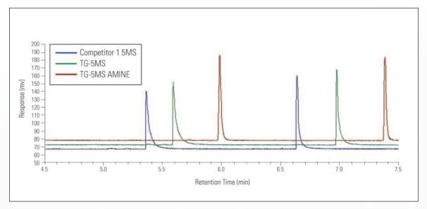
Figure 4: Using the treated TraceGOLD AMINE column substantially reduces the effect of tailing and increases the sensitivity of the assay compared to other columns.
