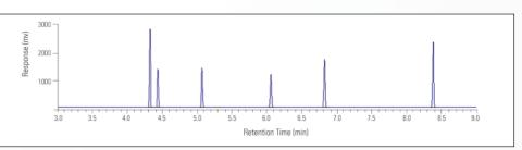
Figure 3: Analysis of a series of phenols using columns made from different batches. The data demonstrates the excellent batch-to-batch reproducibility obtained with the TraceGOLD TG-5MS GC column.
