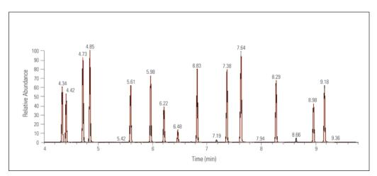
Figure 2: Overlay of 100 chromatograms showing the column robustness over 100 injections, with excellent retention time stability.
