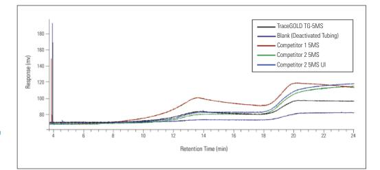
**Figure 1:** Column bleed obtained from TraceGOLD TG-5MS GC column and 4 leading competitors, clearly demonstrating the low bleed characteristics of this column.
