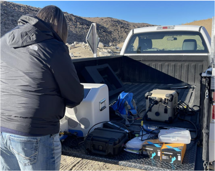
Figure 3. Rear view of the truck used to both approach the blast pits and to perform immediate analysis on the samples collected. The Continuity™ portable mass spectrometer is in the truck bed on the left partially covered by the operator and powered by an external battery on the right. A field operator is seen analyzing the collected samples on-site, demonstrating the capability of the instrument for immediate, in-field analysis. This simple setup highlights the portability and adaptability of the Continuity™ system for rapid deployment in remote and challenging environments.
