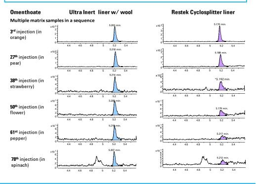
Ultra Inert splitless liners with wool are suitable for different injection modes from HSL, CSL to LVI
